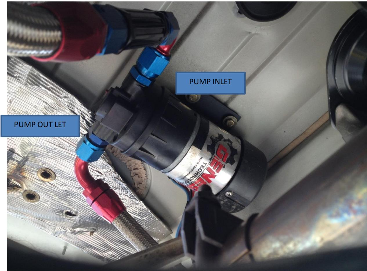
CONNECT ELECTRIC WIRING OF PUMP FOLLOWING INSTRUCTIONS FROM PUMP MANUFACTURE
