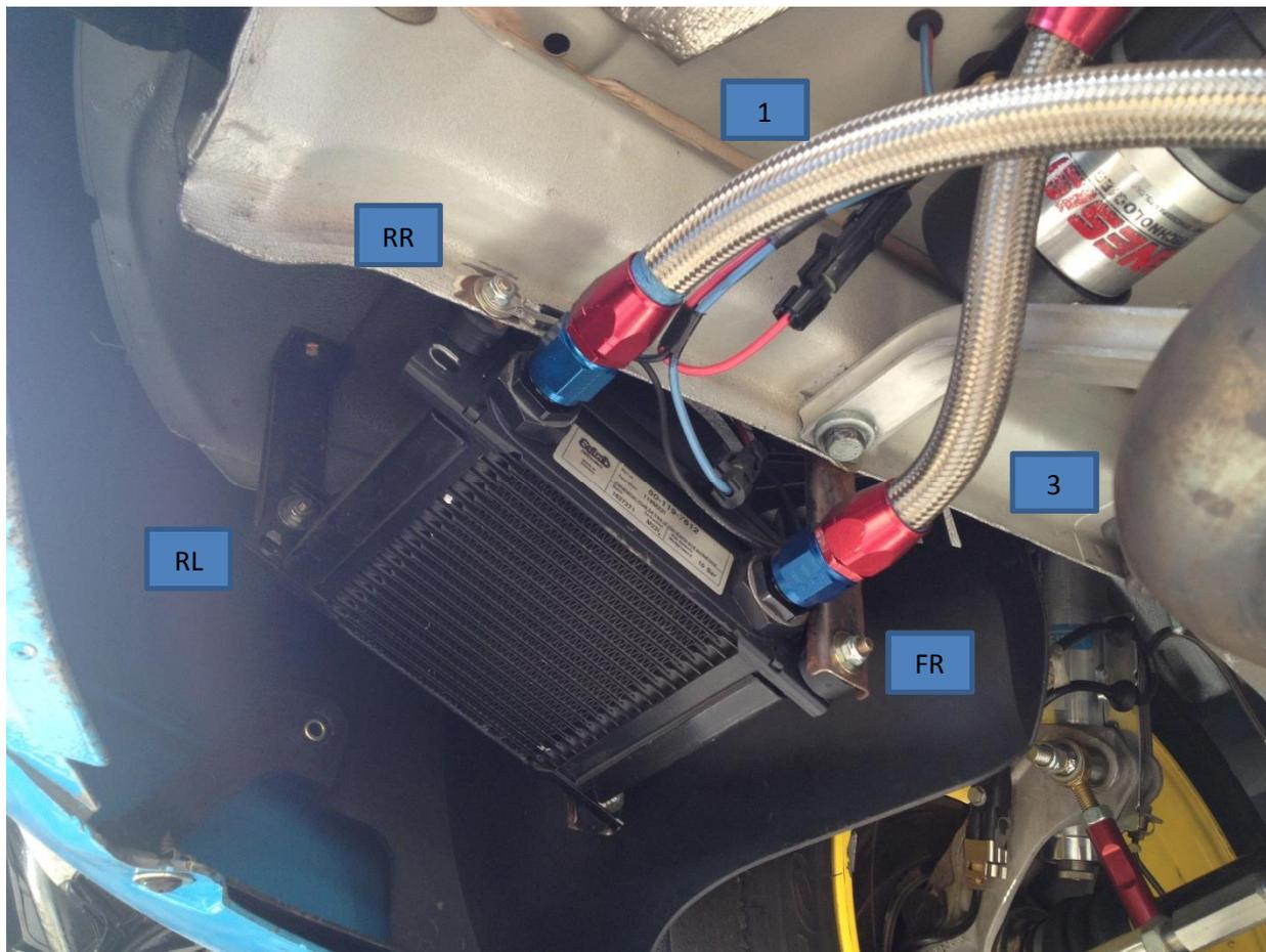
INSTALL (RR) REAR RIGHT BRACKET 4 INCHES FROM REAR EDGE OF VEHICLE
