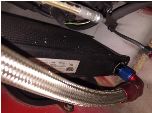
This AN fitting and hose is connected to the furthest port on the cooler and runs directly to the other AN fitting on the heat exchange delete (closest to the back of the vehicle)
