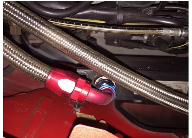
This AN fitting is connected to the back port (closest to the rear of the car) on the cooler and runs directly to the tee-fitting on the remote oil filter adapter
