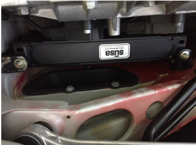
This is the position the oil cooler should sit in in front of the air inlet on the passenger side. Make sure the cooler has the AN fittings on the top of the radiator.
