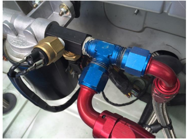
Tee-fitting shown above with the two connections (from accusump, bottom, and from the cooler, right)
