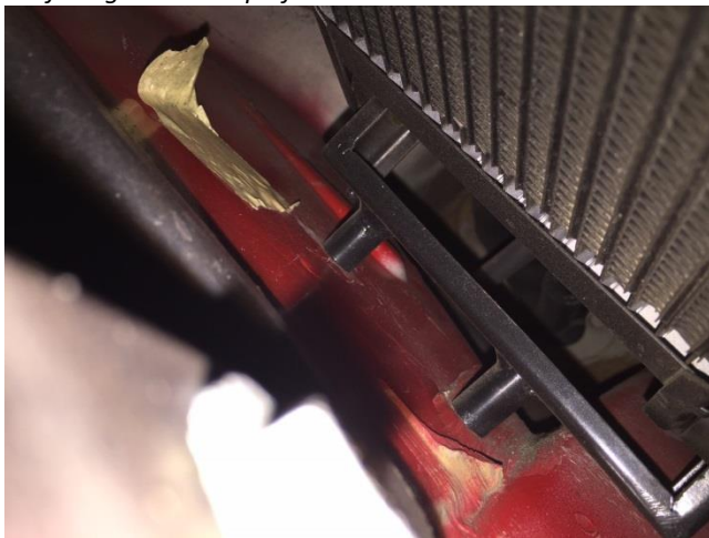
You will need to bolt the brackets to the body by drilling holes and using locking bolts/nuts (not supplied) to secure them in place.
