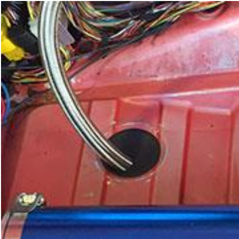
This is where we drill the hole in the rear trunk body for the braided line to be fed through. You can dress it up nicer with a rubber grommet once it's complete.
