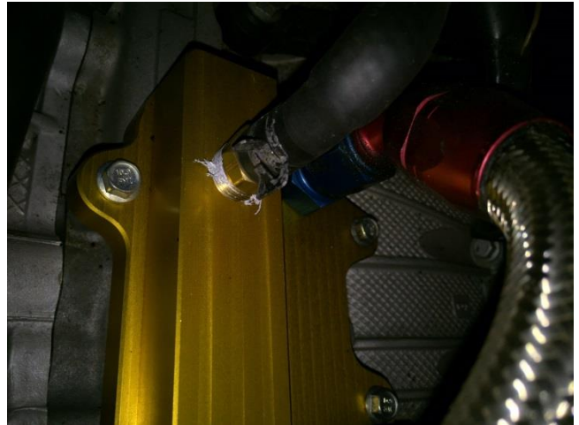
Photo shows the heat exchange delete and where your AN fitting and hose line needs to be connected to from the check valve on the oil filter holder.
