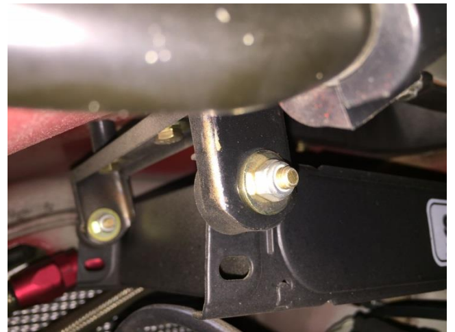
Brackets shown with anti-vibration rubber mounts
