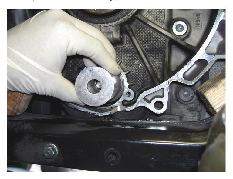
Tap the end of the insertion tool until the bearing is seated completely. You will hear a ‰olid+change in sound when the bearing has reached the engine block.
