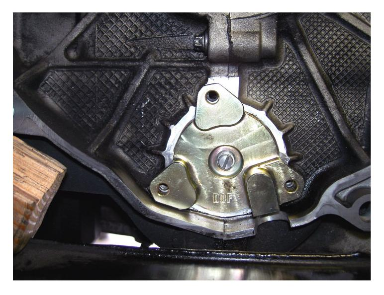
Check the clearance for the DOF/Oil line screw-in adapter on the bell housing cut-out that you made before. Adjust the clearance if necessary with a file.
