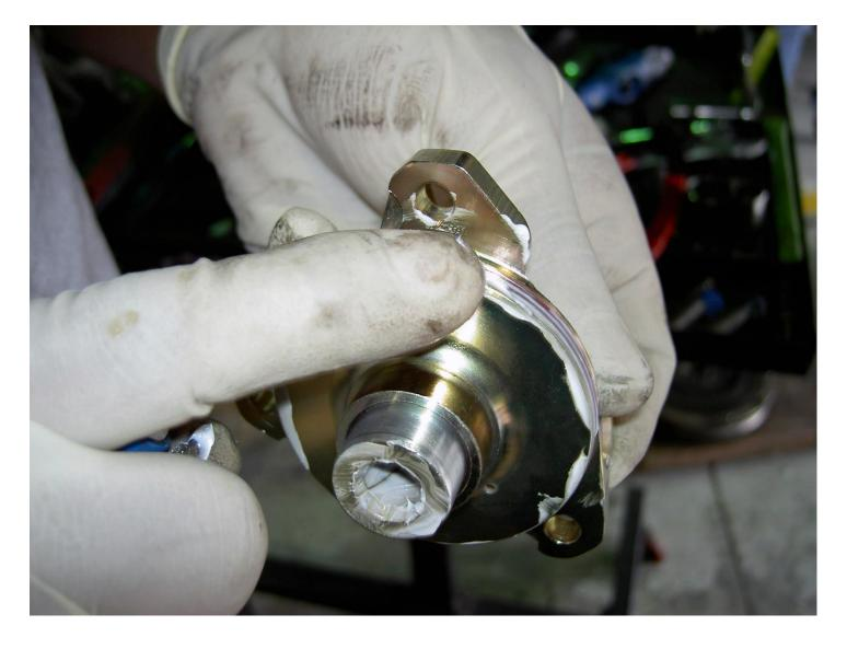
Place the new DOF flange with spacer ring in place onto the bearing support shaft.
