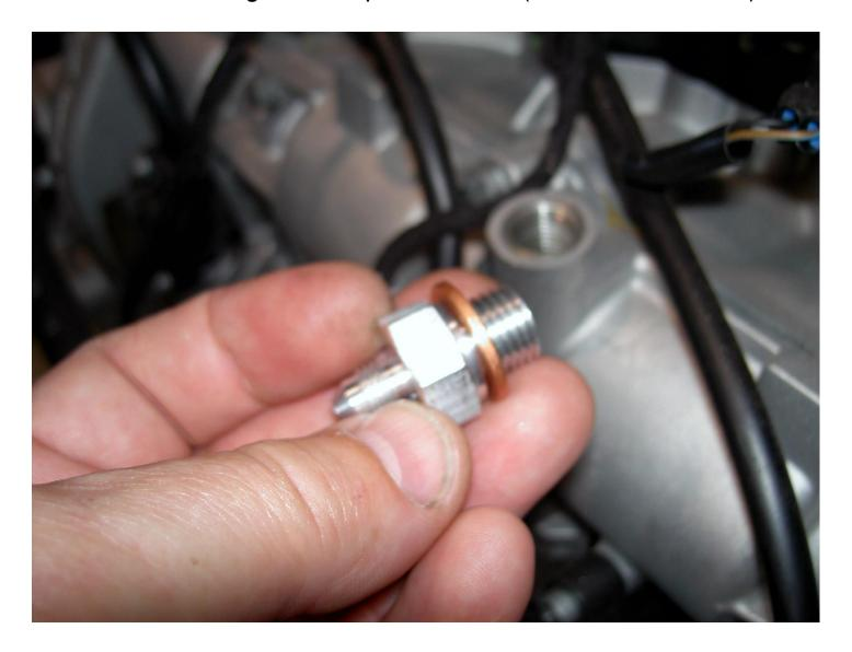
Finally thread the free end of the high pressure oil line onto the newly inserted adapter and torque to 13 Nm (10 lb-ft or 115 lb-in).
