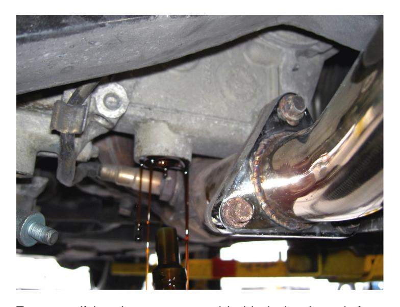
Test to see if there is any movement (slop) in the bearing shaft. Lateral movement (slop) means that the bearing has started to wear down. We recommend that a new bearing be installed regardless, but if the existing bearing is not going to be replaced, remove its outer seal using a sharp pick or small screwdriver and proceed to the %REPARE AND INSTALL DOF FLANGE+step, further down in these instructions.
