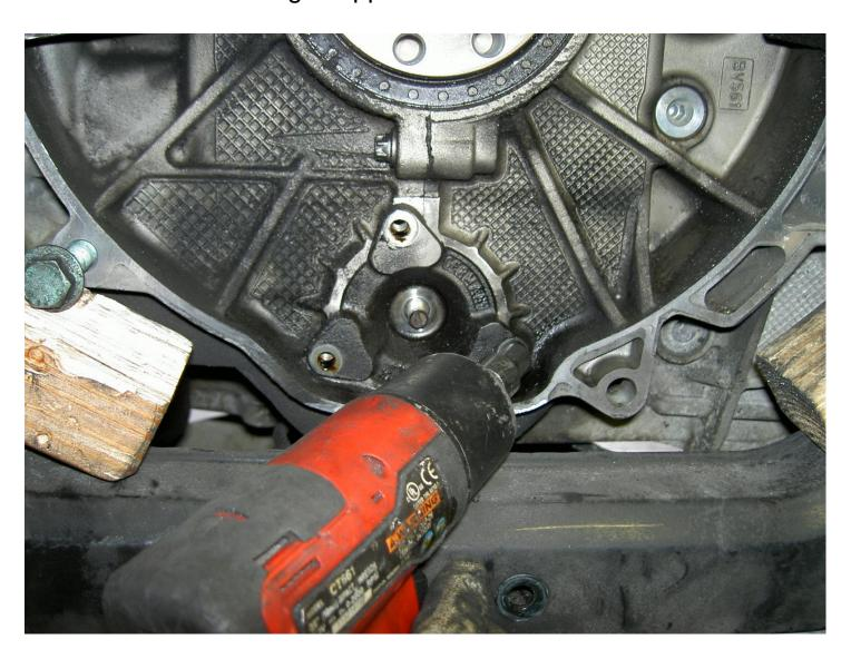
Using a couple of flat-bladed pry bars or strong screwdrivers slowly and carefully pry out the existing bearing flange.
